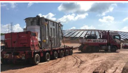
We transported one unit of 45 MVA Power Transformer along with its accessories from Port Klang to Kuala Muda, Kedah for a 40MW solar plant.
